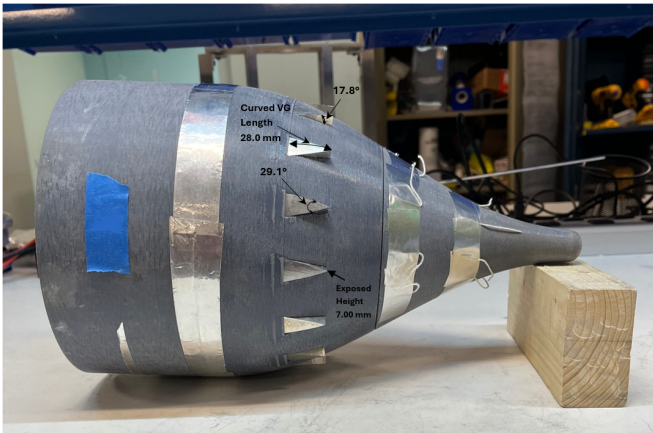
Fig. 9: Dimensions for Tail 3, best performing configuration in terms of drag reduction. See Appendix for tabulated values.
