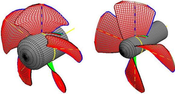
**Figure 6.** 3D geometry rendering: (left) *old* propeller, (right) *new* propeller. Since the present implementation of OpenProp does not treat propeller skew, these 3D renderings are skew-free, although skew was used in the *old* propeller design.
