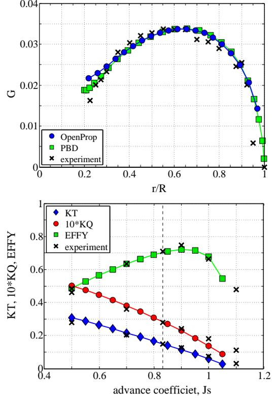
**Figure 3.** (top) Design circulation distribution for U.S. Navy propeller 4119. (bottom) Performance curves for propeller 4119. OpenProp results agree with PBD code solution and experimental data from [Black 1997].
